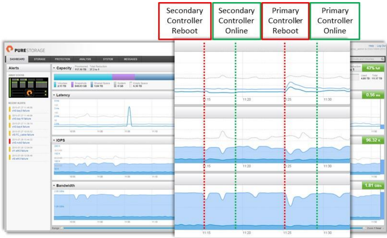
Figure 14. Error Injection Testing—Controller/Software Upgrade Simulation
