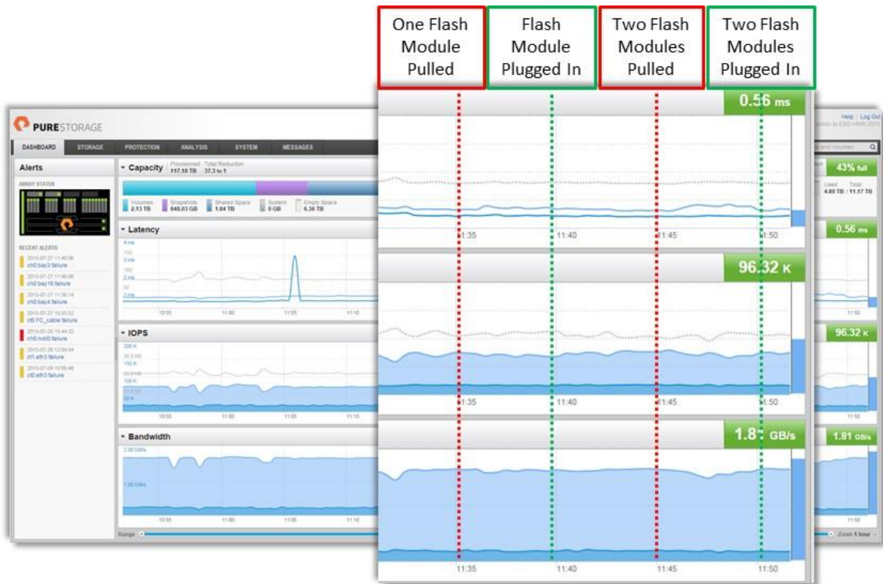
Figure 15. Error Injection Testing—Pulling Multiple Flash Modules
