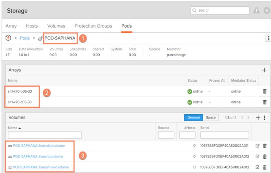
FIGURE 48. Pod connected to both FlashArrays
