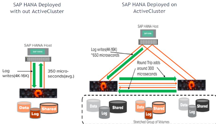
FIGURE 55. Write latency difference with and without an active cluster
