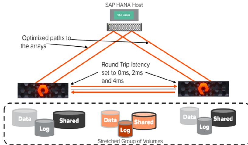
FIGURE 56. Optimized paths to both arrays
