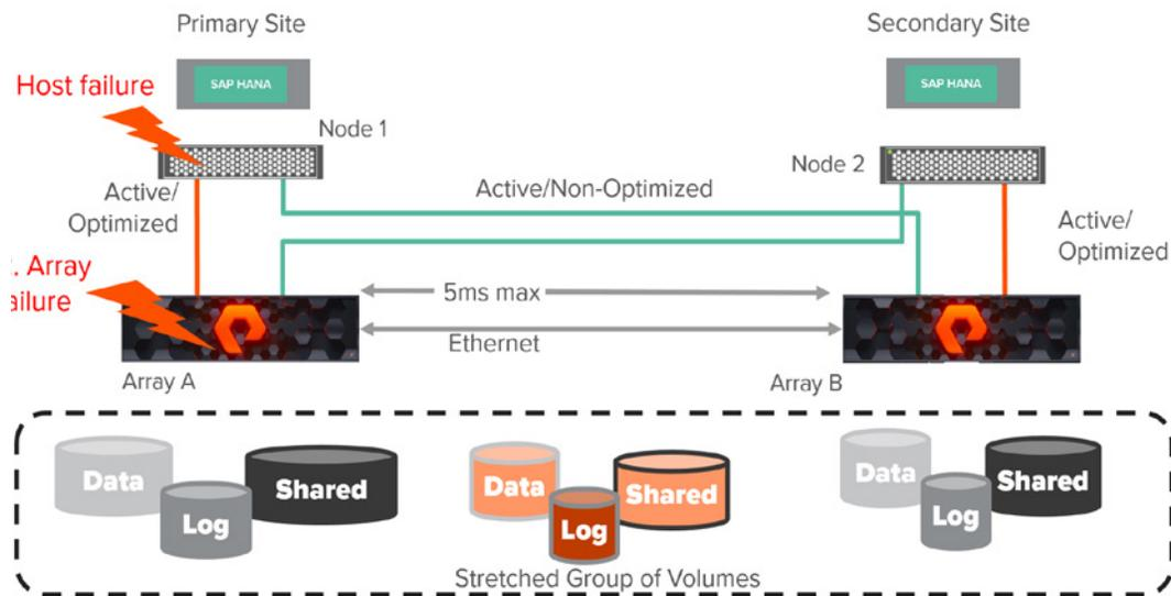
FIGURE 58. Remote Disaster Recovery diagram
