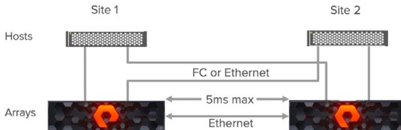
FIGURE 6. Logical paths between hosts and arrays
