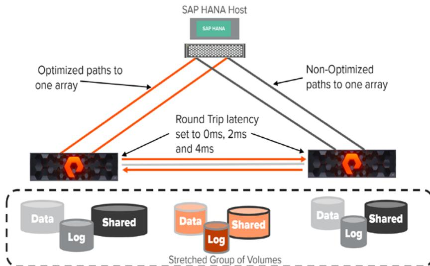
FIGURE 57. Optimized/non-optimized paths to both arrays
